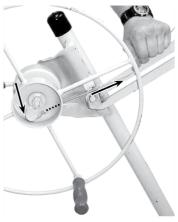
**9.** Feed the crimped end of the cable through the hole in the winch drum and secure it behind the mooring tab by hand pulling the cable snug as shown.
