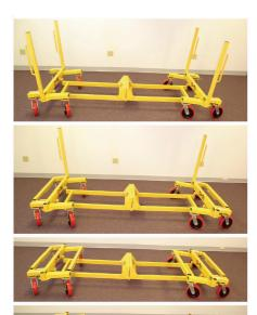
The support arms can be installed in a wide variety of positions depending on the support needs of the load being carried.
