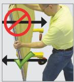
**5.** The support arms can be positioned to configure the Troll® Cart for use as a flatbed cart.
